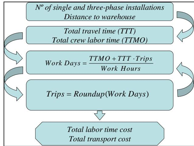
Fig. 6: Installation cost model.
